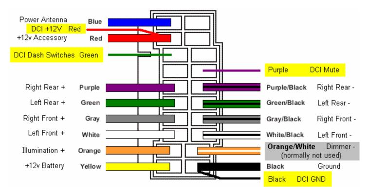
Connections for the DCI are highlighted with a yellow background and connect to the DCI harness only - match them by color. Other wires do not necessarily match by color. All connections to your head unit must be matched by FUNCTION, which may not follow the 'standard' color code shown in the above diagram. See the notes below and refer to the wiring diagram supplied with your head unit to verify all connections.
